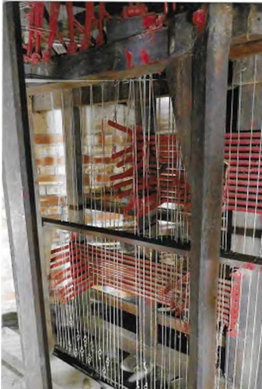
Fig. 33. Part of the transmission between the carillon machine and the bells. Photo by Paul-Félix Vernimmen, grandson of Séverin van Aerschodt, reproduced by kind permission of the Grosvenor Estate.
