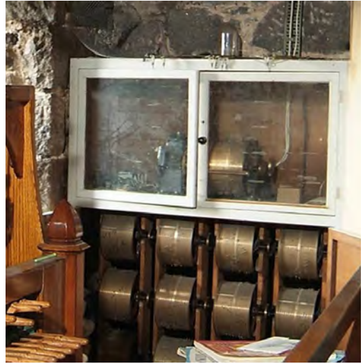
Fig. 40. There are two sets of nine tune barrels, one of which is illustrated here, mounted below the automatic carillon machine. This set has secular tunes and the other, which is out-of-shot has sacred tunes. They have not been played for several years now.
