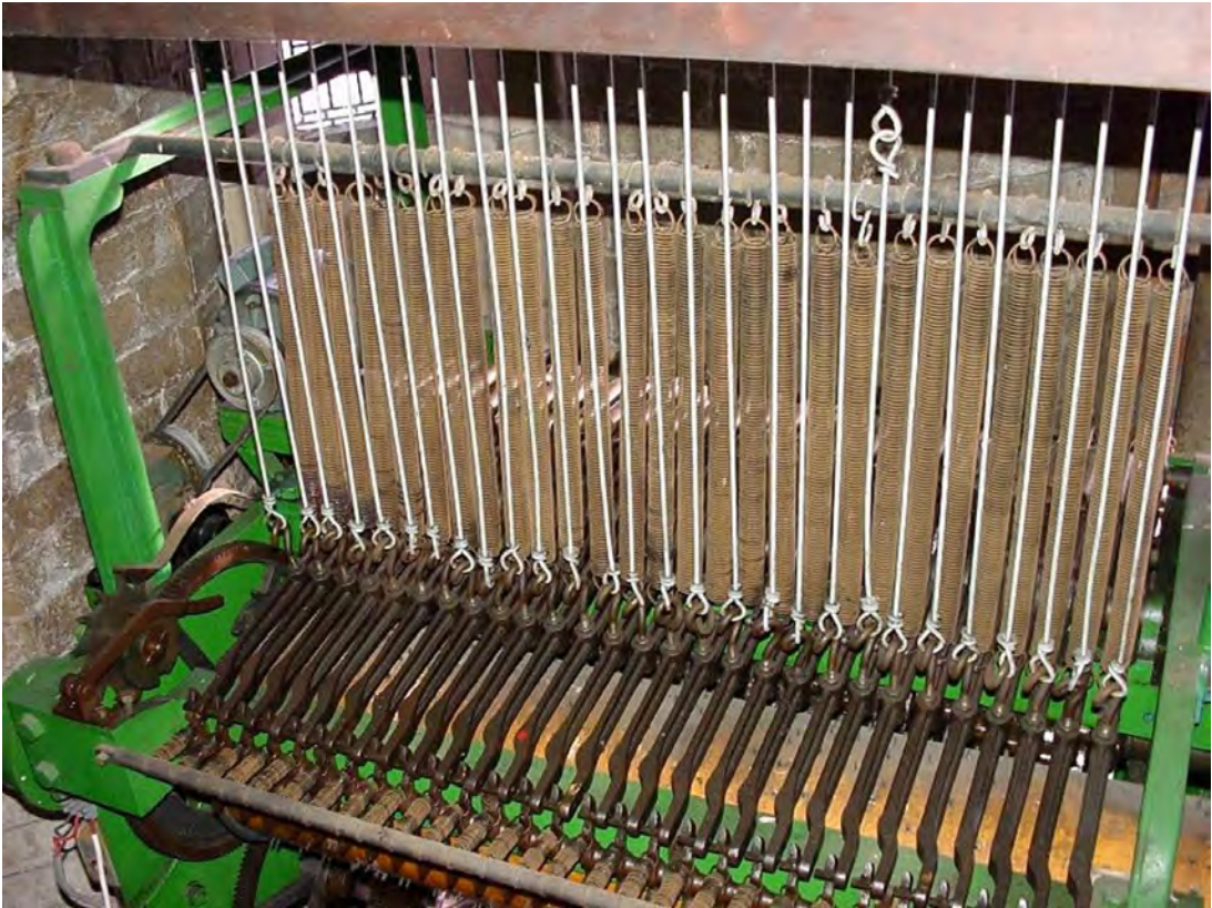
Fig. 31. Eaton Hall carillon machine detail. This shows the upper left-hand half of the carillon machine and part of the pinned drum beneath; the lightweight triggers in front of the drum are tripped by the pins allowing the hammers to drop and are then immediately raised again as in the Imhof system mentioned earlier. Photo by Steve Thomas, reproduced by kind permission of the Grosvenor Estate.
