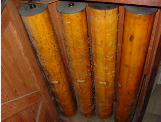
Fig. 32. Four of Eaton Hall's tune barrels are stored in a cupboard; the makers claimed that they could be changed by one man with little effort. One of the barrels (on the right) appears to have space left for more tunes to be pinned on it if required. Photo by Steve Thomas, reproduced by kind permission of the Grosvenor Estate.
