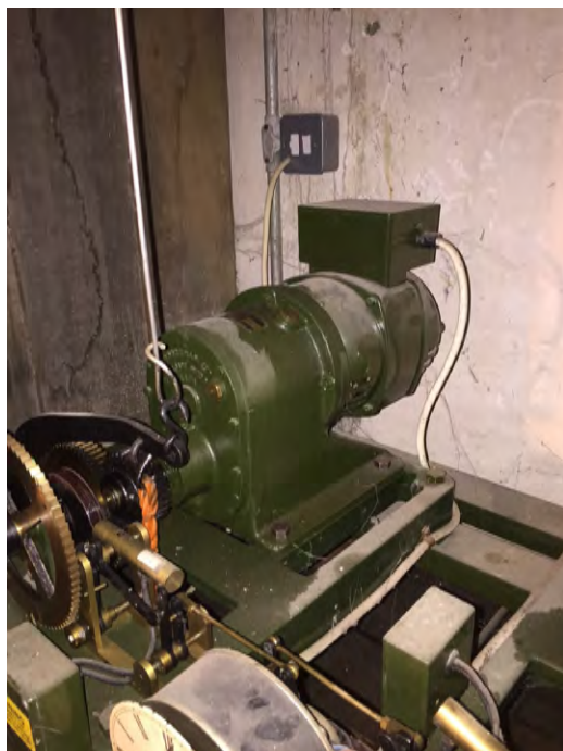
Fig. 23. At an unknown date in the twentieth century the clock was converted to direct electric drive by AC motors, by persons unknown. This image shows the strike train. Image thanks to Cumbria Clock Company.
