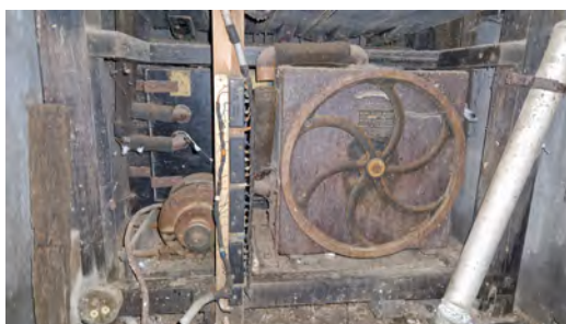
Fig. 18. Adjacent to the G&J clock is a now unused vacuum-pumped chiming apparatus. This must have been controlled from a now missing keyboard or punch card machine as in fairground organs. There are fifteen levers at the back, but no longer any linkages to the bells. A faint pressing indicates a date of 1952.
