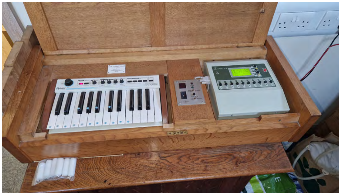
Fig. 20. The chimes are now controlled from a John Taylor & Co keyboard and an Apollo controller produced by the Belgian company Clock-o-matic, both of unknown dates. This also functions as a clock and sets off the hour strike and quarter chimes.
