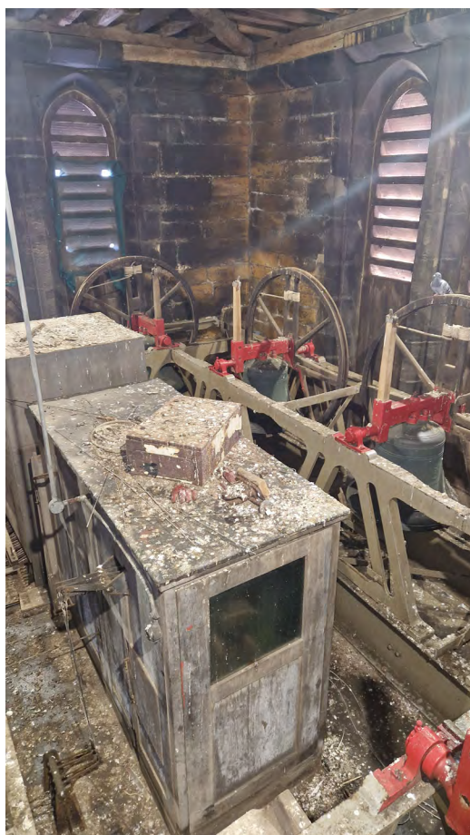
Fig. 20. The chimes are now controlled from a John Taylor & Co keyboard and an Apollo controller produced by the Belgian company Clock-o-matic, both of unknown dates. This also functions as a clock and sets off the hour strike and quarter chimes.
