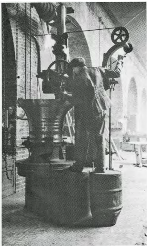
Fig. 8. The vertical tuning lathe at the Van Aerschodt foundry. Image thanks to Paul-Félix Vernimmen, 1982, and Chris Pickford.
